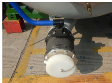
Figure 3: 6" URT Product discharge line
