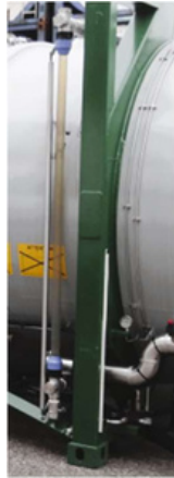
Figure 12: Sight Glass, observe product fill levels
