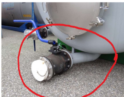
Figure 18: 6" URT product discharge connection
