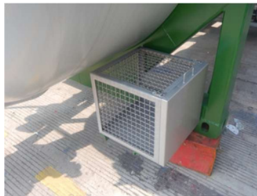
Figure 6: Cage for storage of fittings during transport
