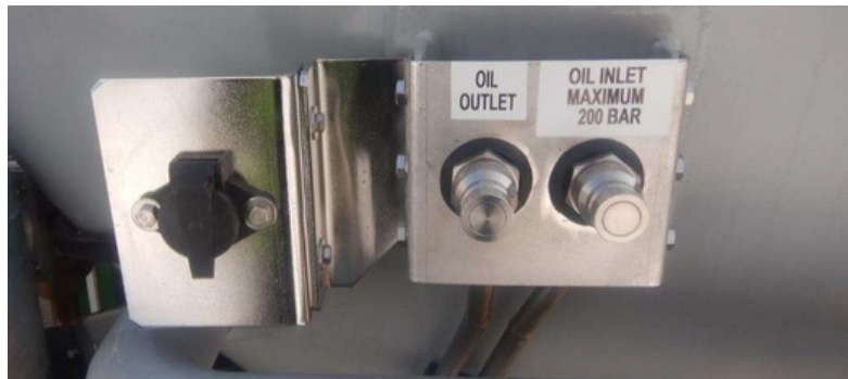
Figure 8: Hydraulic hose connections and control switch
